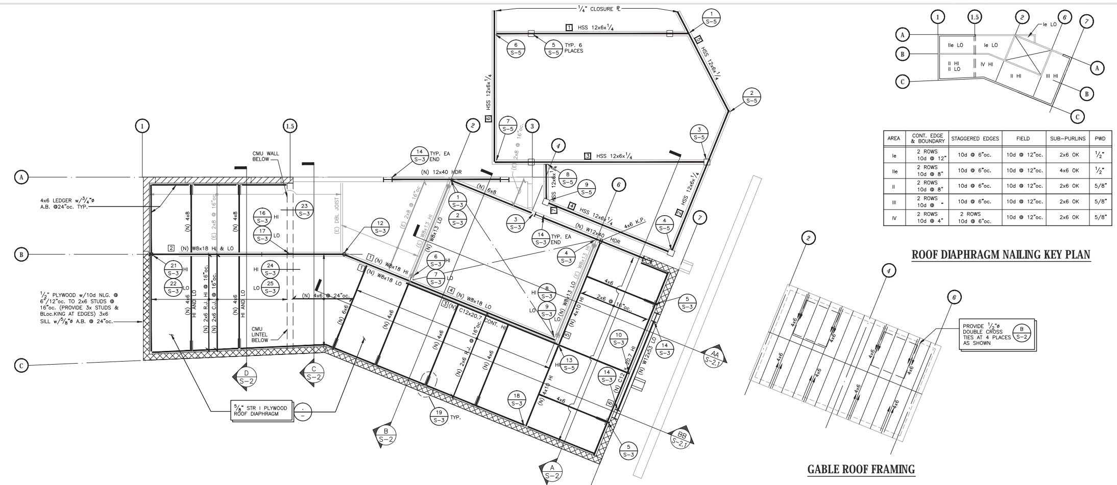
ROOF FRAMING PLAN
